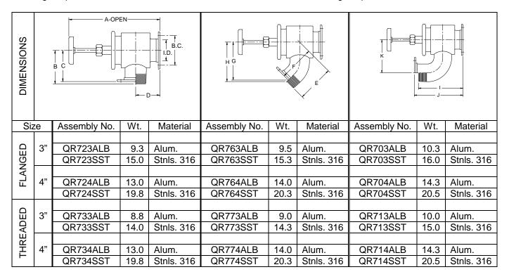
NOTE: Stainless 316 valves are standard with Teflon disc, gasket & packing (Suffix "T"). Aluminum valves are standard with Buna-N disc, cork-buna-N gasket and Teflon packing (Suffix "B"). For variations and replacement parts see section 10, page 5B.
