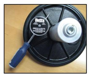
The new vent body does not have wrench flats for gripping during installation, but a standard screwdriver can be inserted through the cross-drilled hole in the vent for tightening. This method of installation will not damage the vent but care should be used not to excessively tighten the vent. A similar method can be used to un-install the vent.
