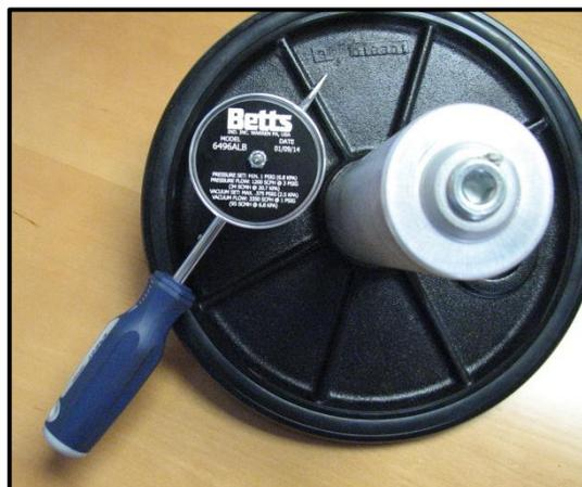
The new vent body does not have wrench flats for gripping during installation, but a standard screwdriver can be inserted through the cross-drilled hole in the vent for tightening. This method of installation will not damage the vent but care should be used not to excessively tighten the vent. A similar method can be used to un-install the vent.
