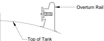
NOTE: The above is not intended to be a recommendation that overturn rails be used for conduits in vapor recovery system or that vent must be mounted as shown. It merely shows one type of mounting to illustrate that clearance is needed for the spring end of vent to insure proper operation.
